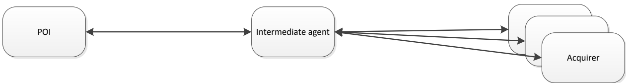
FIGURE 45: INTERMEDIATE HOST CONNECTED TO SEVERAL ACQUIRERS
